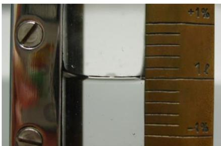
Figure 1. Standard test measure meniscus
